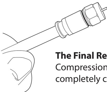
**The Final Result:** Compression Connector completely compressed
