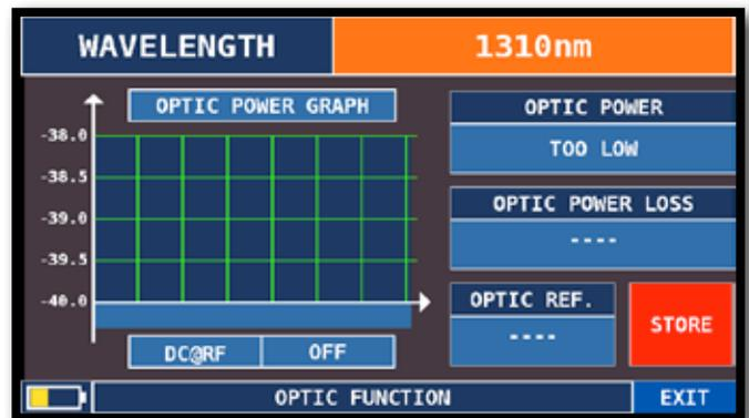
Touch “WAVELENGTH” and select the required wavelength, for example 1310 nm
