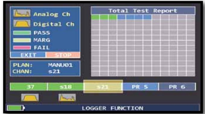
Touch "SAVE DATALOGGER" and set the parameters required. Touch "START SAVE" to create a new log file
