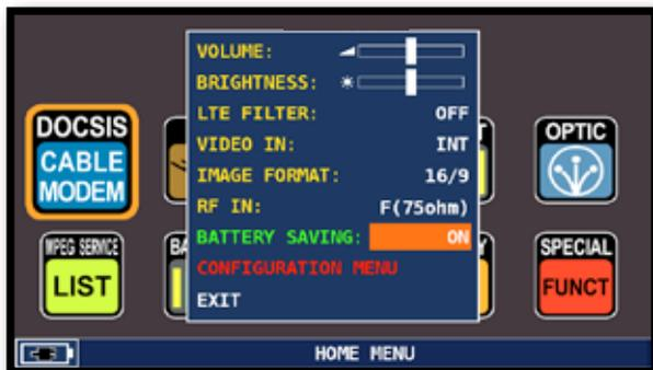
Choose "BATTERY SAVING" from the volume screen. In ON mode, if no key is pressed, after 30 seconds, the display brightness is reduced and after 5 minutes the meter automatically turns off. Press any key to temporarily reset the battery save mode.
