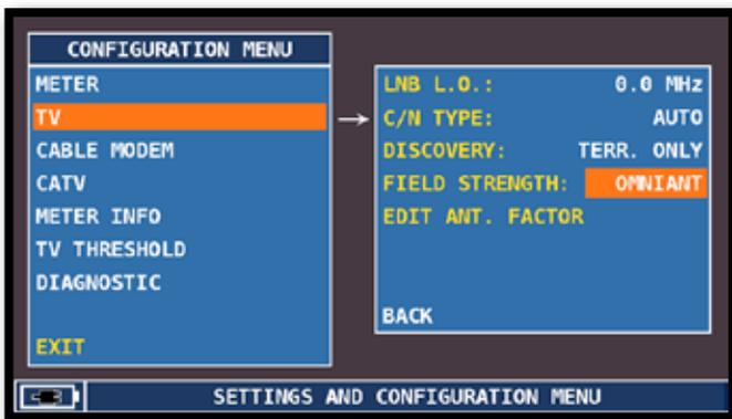
Touch "Field Strength" and select the antenna model: "OMNIANT, LOGANT or CUSTOM"
