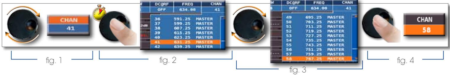
How to select the frequency and set the value using the numerical keyboard:
