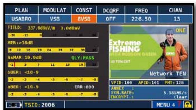
Press the TV key: The field strength is shown on the right of the "POWER" measurement
