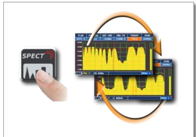
Press to cycle through spectrum analyzer screens
