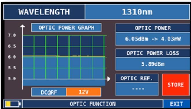
Touch “DC@RF” and select, if it is required, the power supply voltage: for example 12V.
