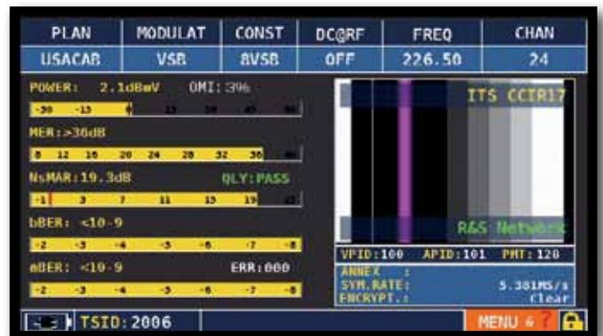
Press the "TV" key to carry out the RF measurements & OMI
