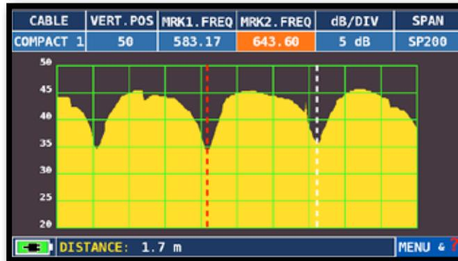
In the DISTANCE window, read the cable's mismatching value: example 1.7 m
