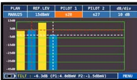
Touch "PILOT 1" and "PILOT 2" to select the two channels to be used for the tilt measurement (level difference)
