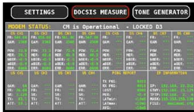
The meter will start scanning the selected channels in order to connect to the CMTS. While performing this process the display will indicate Scanning now at bottom and WAIT or UNLOCKED in the various parameters fields. Once completed the synchronization process, the LCD will display "CM is Registered" and will report a summary of the major information about the active connection:
