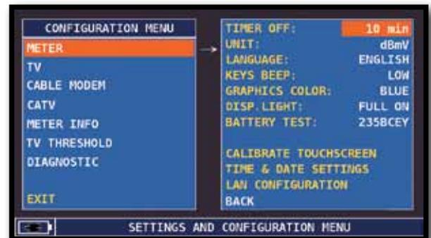
Touch "CONFIGURATION MENU", then "METER" in the volume screen, and set the "TIMER OFF" value required. The meter will turn off after 5, 10, 15 or 30 minutes of inactivity. Press any key to interrupt the automatic turn-off.
