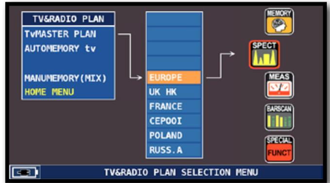
In TV or CATV mode press the "PLAN" key, select the plan required, then "SPECT" to visualize the spectrum
